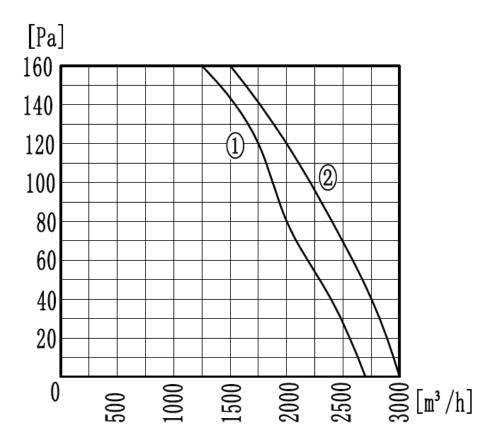
Curve 1: 50HZ Curve 2: 60HZ
